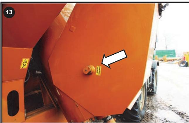
Grease Discharge Auger spout (Both sides)
