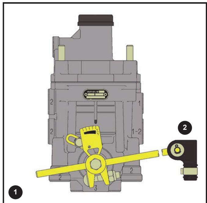
The service pressure may be modified by the RELSV (1) based upon the physical load sensed by the valve, as weight is removed from the trailer its chassis rises, causing the RELSV (1) operating arm to lower (rotate clockwise).
