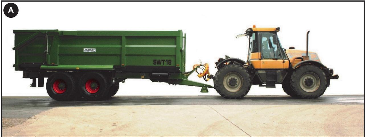
Adjust the drawbar and/or the hitch of the towing vehicle so that when towing the trailer body is parallel to the road surface.
