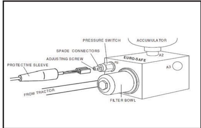
**Note! The pressure switch is factory set and sealed. If seal is broken warranty for the unit becomes void.**
