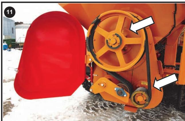
Grease Auger drive belt pulleys
