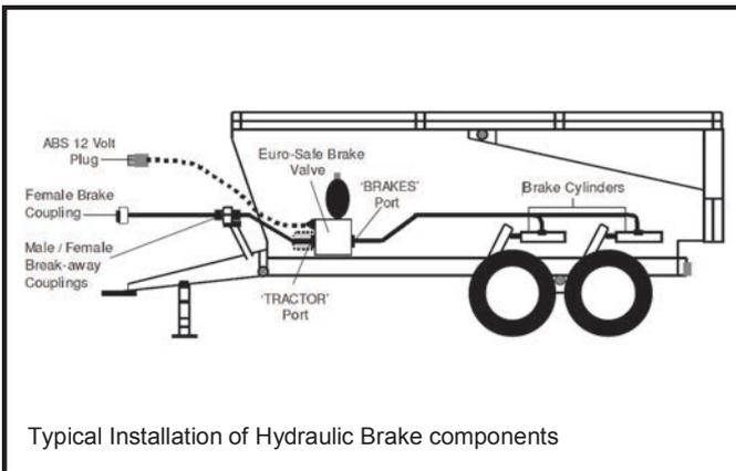
Typical Installation of Hydraulic Brake components
