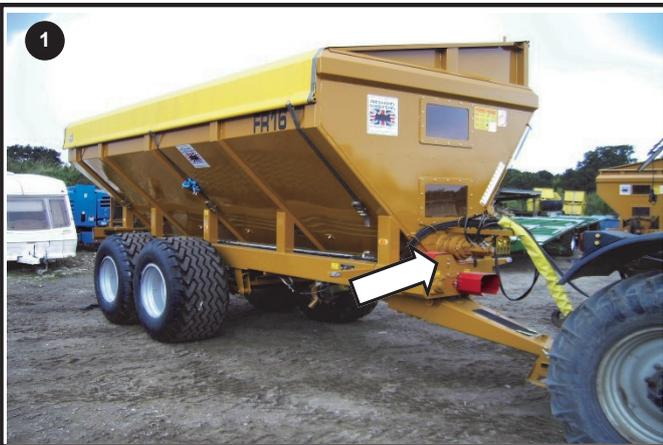
Check All Air and Hydraulic Lines for signs of Damage
