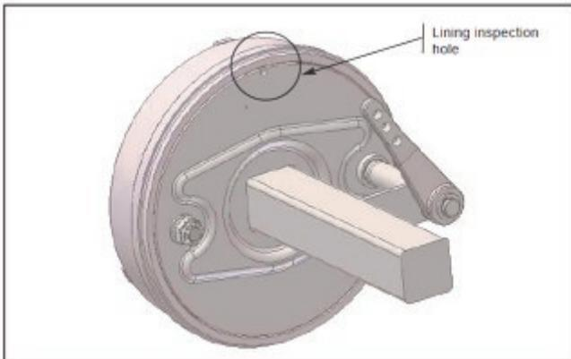
as the minimum lining thickness is reached.
