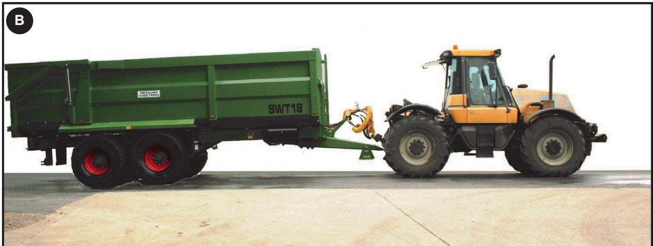
Hitching too high will cause unnecessary wear to the suspension and brake components of the rear axle, and reduce the braking efficiency. It can also cause stability problems for the trailer and towing vehicle
