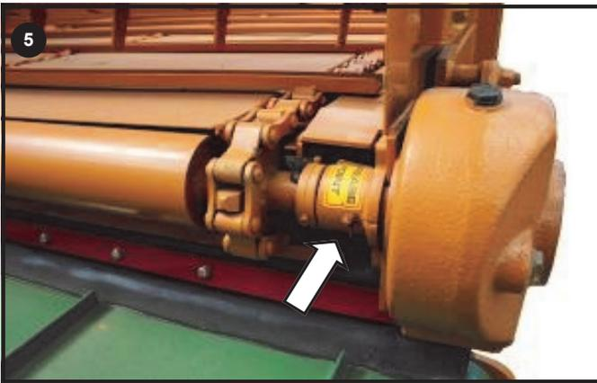
Grease Left Side Floor Drive shaft Support Bearings
