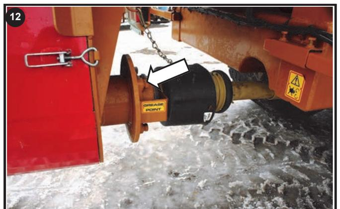
Grease Lower pulley shaft (Two positions)
