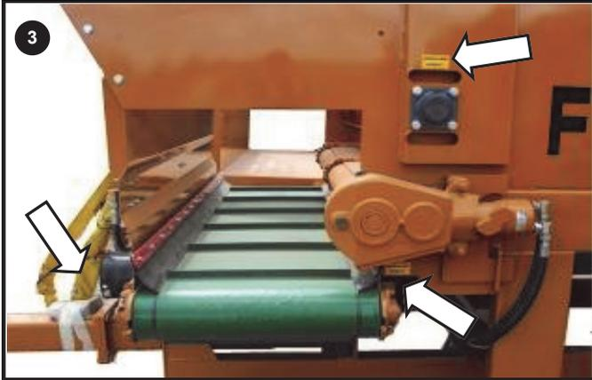
Grease Left and Right side Conveyor Support Bearings & Lower Beater support bearing
