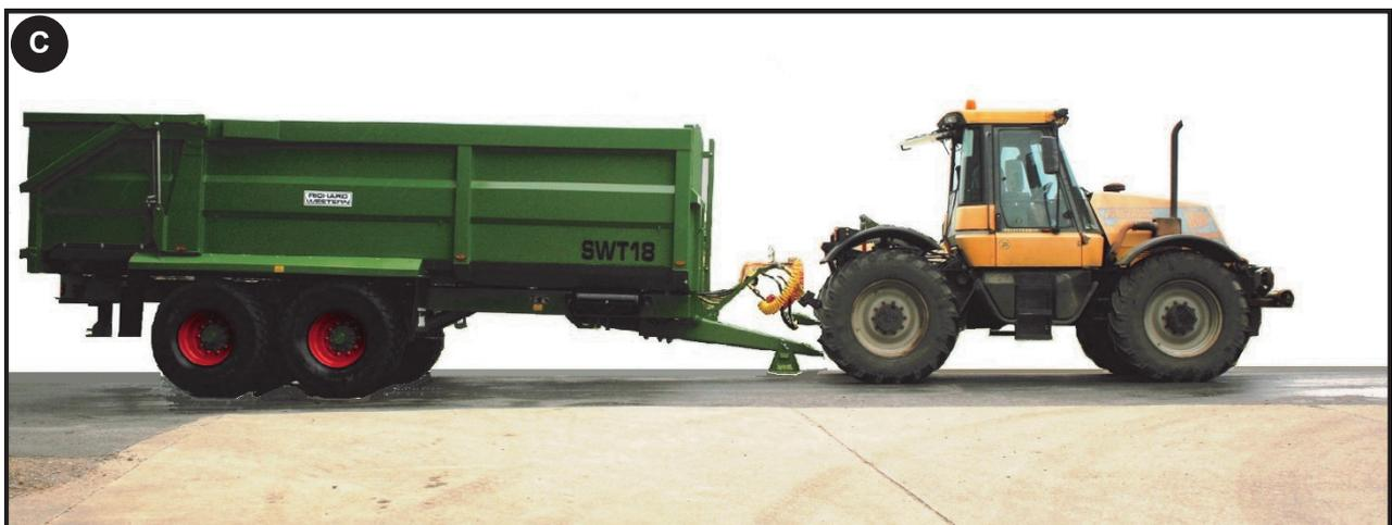
Hitching too low will cause unnecessary wear to the suspension and brake components of the front axle, and reduce the braking efficiency. It can also cause additional loading to be placed on the towing vehicle, possibly causing damage to rear axle and brake components.
