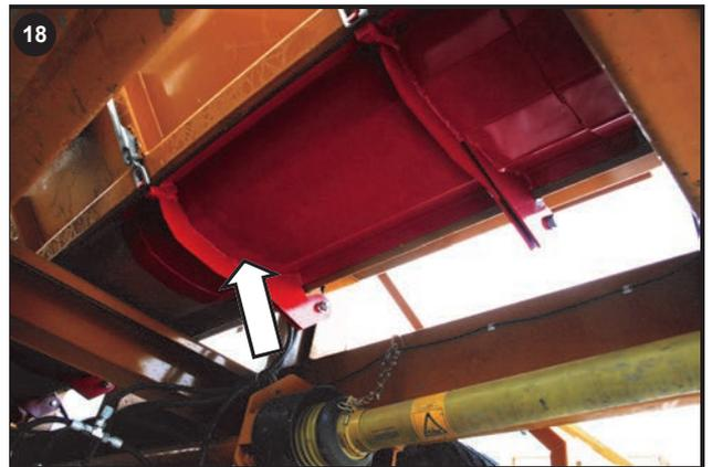
Grease Mid Auger bearing (Open Clear out hatch)
