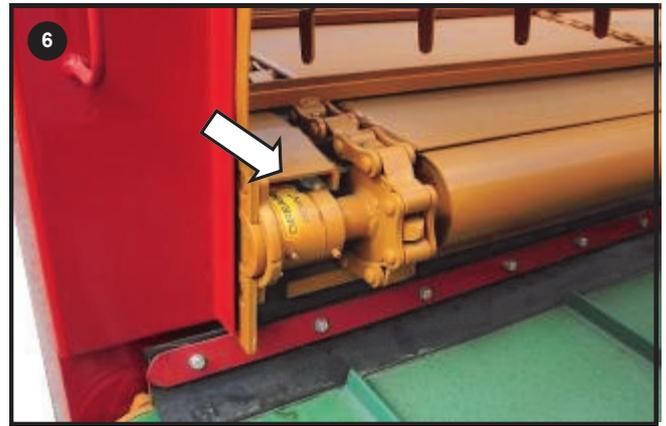
Grease Right Side Floor Drive shaft Support Bearings
