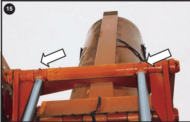
Grease Discharge Auger cylinders
