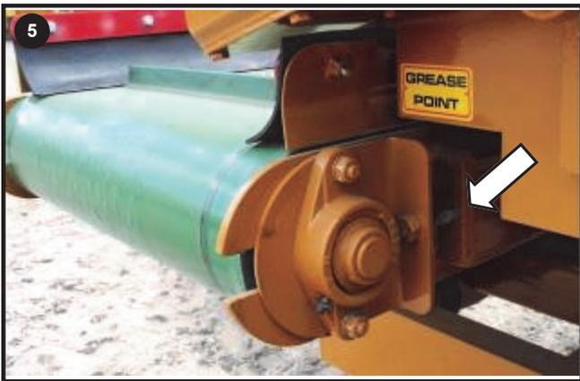
Adjust conveyor evenly to ensure accurate tracking
