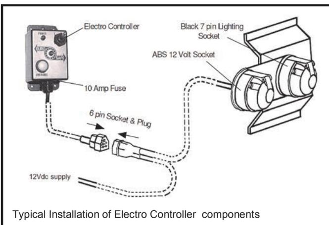
Typical Installation of Electro Controller components
