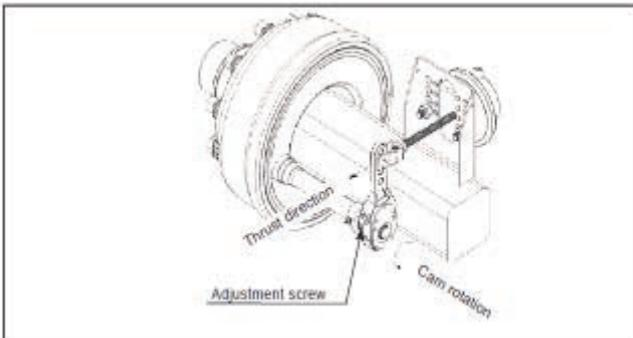
To take up the slack, turn the adjustment screw on the lever to adjust the relative position of the cam and the lever
