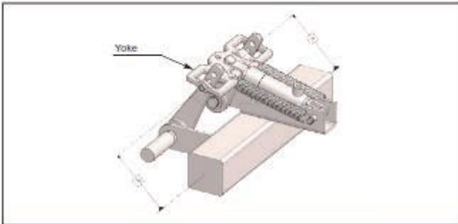
For braking systems which use a yoke, the yoke must remain parallel with the axle especially when the brakes are fully applied. This means that the stroke of the levers on the brakes at each side must be identical. Otherwise, the brake slack must be adjusted.
