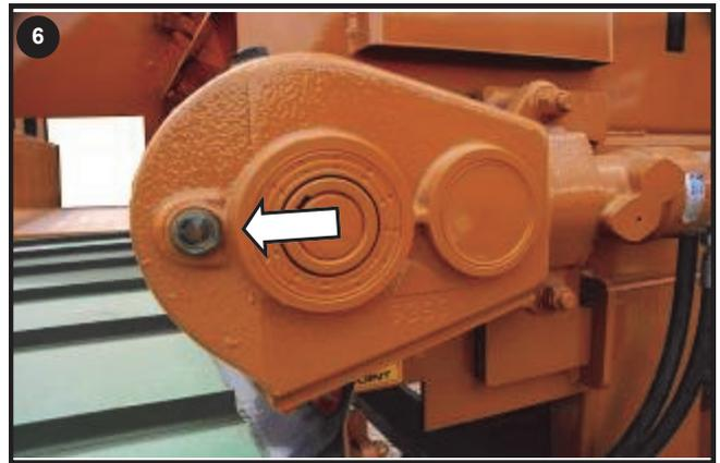
Check drive gearbox oil level. Replenish as required
