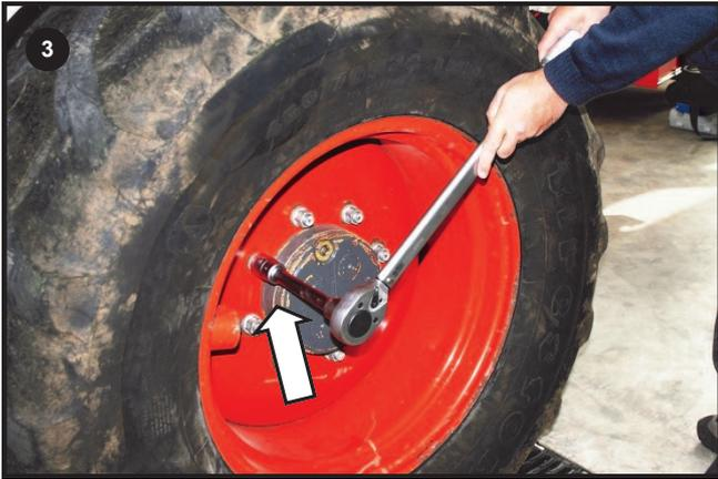
Check Wheel Nut Torque
