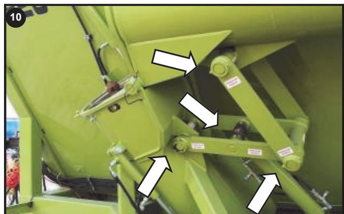
Grease Elevator linkage shafts
