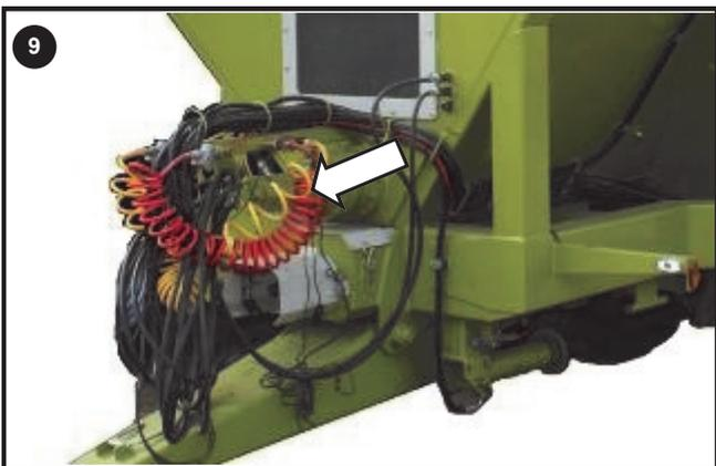
Grease Floor Chain & Check Oil in Drive Gearbox
