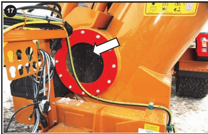
Grease Horizontal bearing (Via viewing window)
