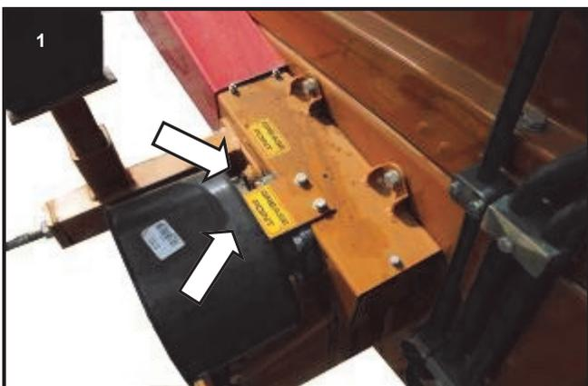
Grease the PTO bearing and the transfer gear support bearing.
