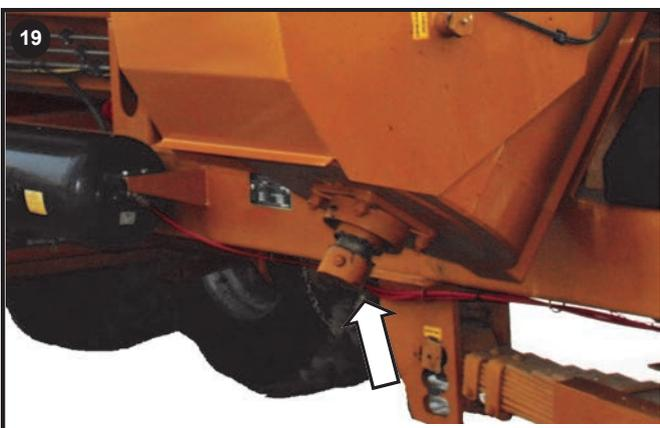
Grease Top Bearing. (Grease internal sliders when stowed)
