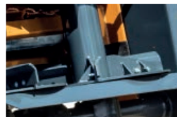
Disc rotor base with three blades on 1100mm rotors
