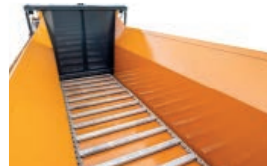
2 heavy-duty floor chains with individual tensioning, 16mm or 20mm, floor slats every 5 links
