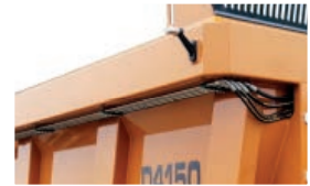
Hydraulic services carried in rigid pipework to reduce maintenance
