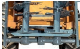
1.7m or 2.0m wide rotor spreading deck
