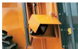
Automatic light protectors with slurry door option
