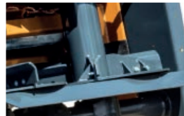
Disc rotor base with three blades on 1100mm rotors
