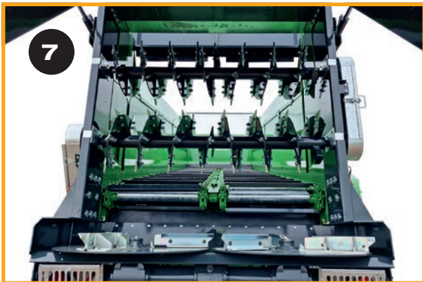
Replace the rotor blades when they become worn to prevent damage to auger See procedure below .
