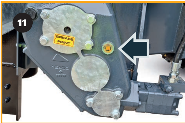
Check Floor Drive Gearbox oil level & top up as required.
