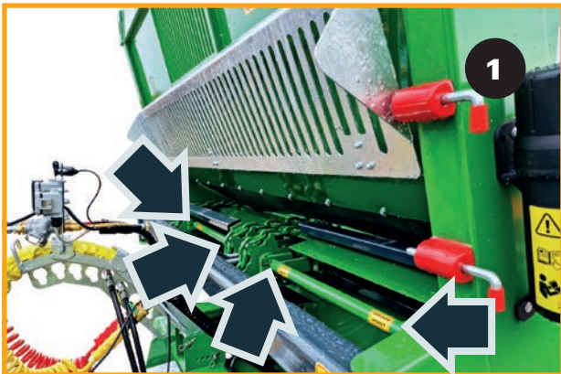
Lift Cover and Grease idler shaft bushes (4 Off).
