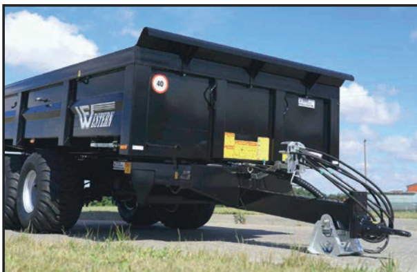
Towing eyelet is mounted in lower position.
