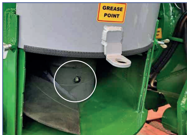
When the shaft is turned, the lubrication points are visible
