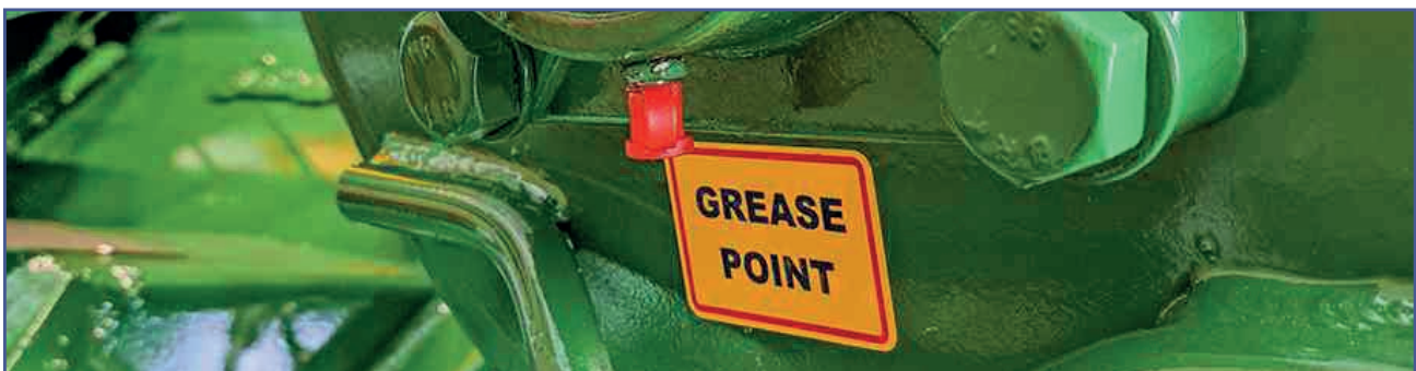
The fifth lubrication point is in the upper part of the vertical discharge auger
