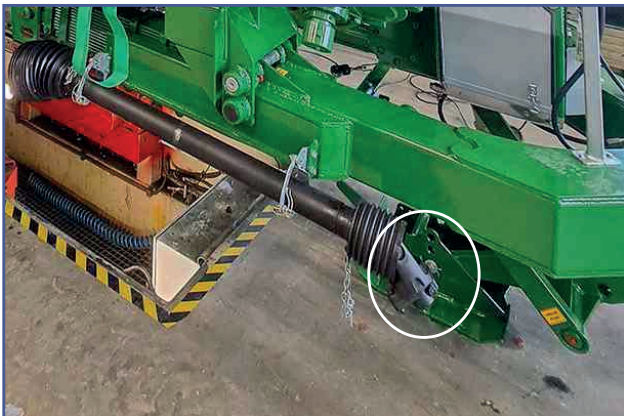
The security shear screw on the PTO.
