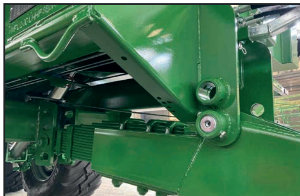
Longitudinal spring drawbar height adjustment.
