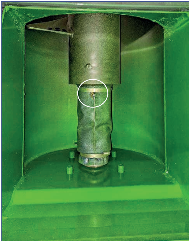
The fifth lubrication point is in the upper part of the vertical discharge auger
