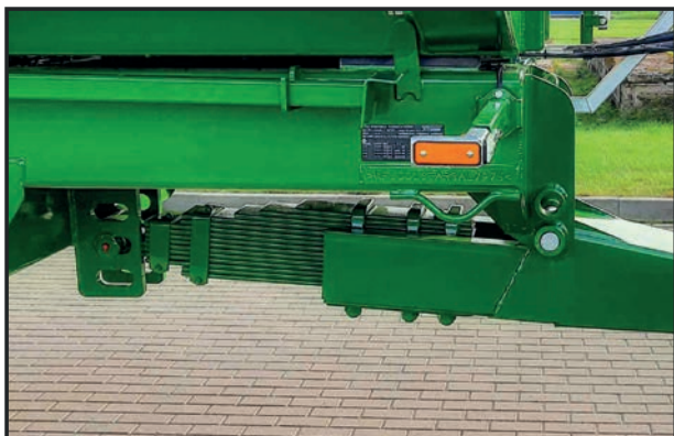
Drawbar with longitudinal spring.
