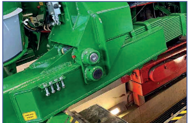
Storage location of the security shear screw.
