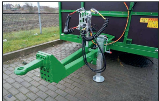
Towing eyelet is mounted in top position.
