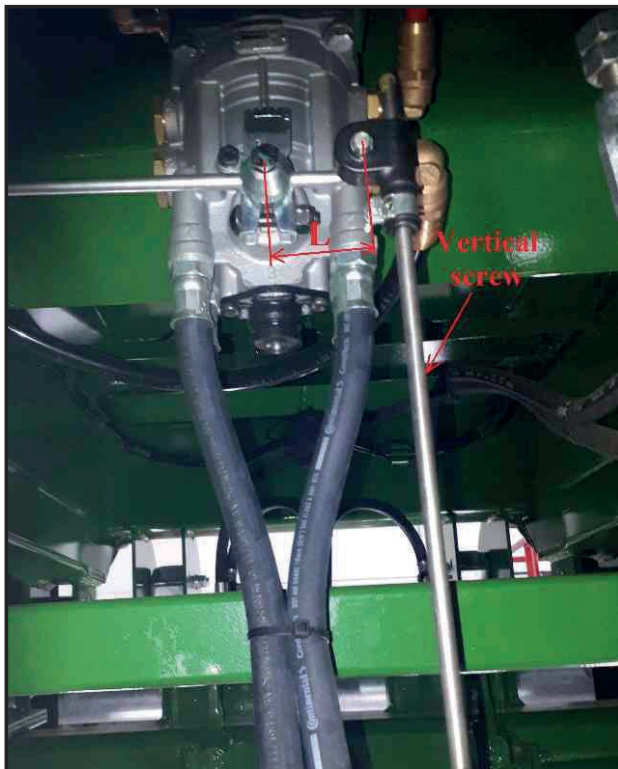
Adjustment for Automatic Load sensing Valve Air Brakes
