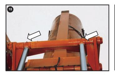
Grease Discharge Auger cylinders
