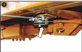
Grease Parking Brake Mechanism
