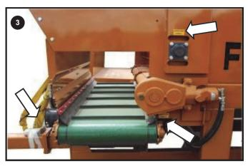
Grease Left and Right side Conveyor Support Bearings & Lower Beater support bearing
