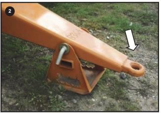
Check the condition of the Towing eye for signs of wear or damage
