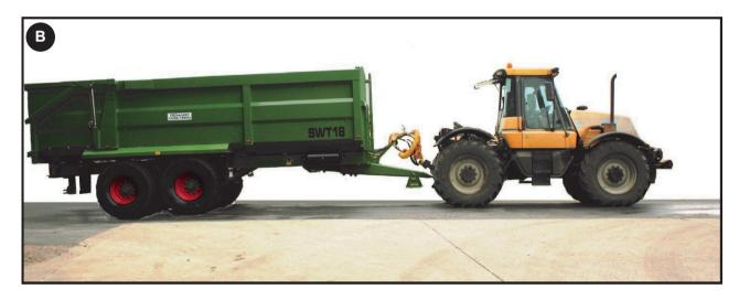
Hitching too high will cause unnecessary wear to the suspension and brake components of the rear axle, and reduce the braking efficiency. It can also cause stability problems for the trailer and towing vehicle
