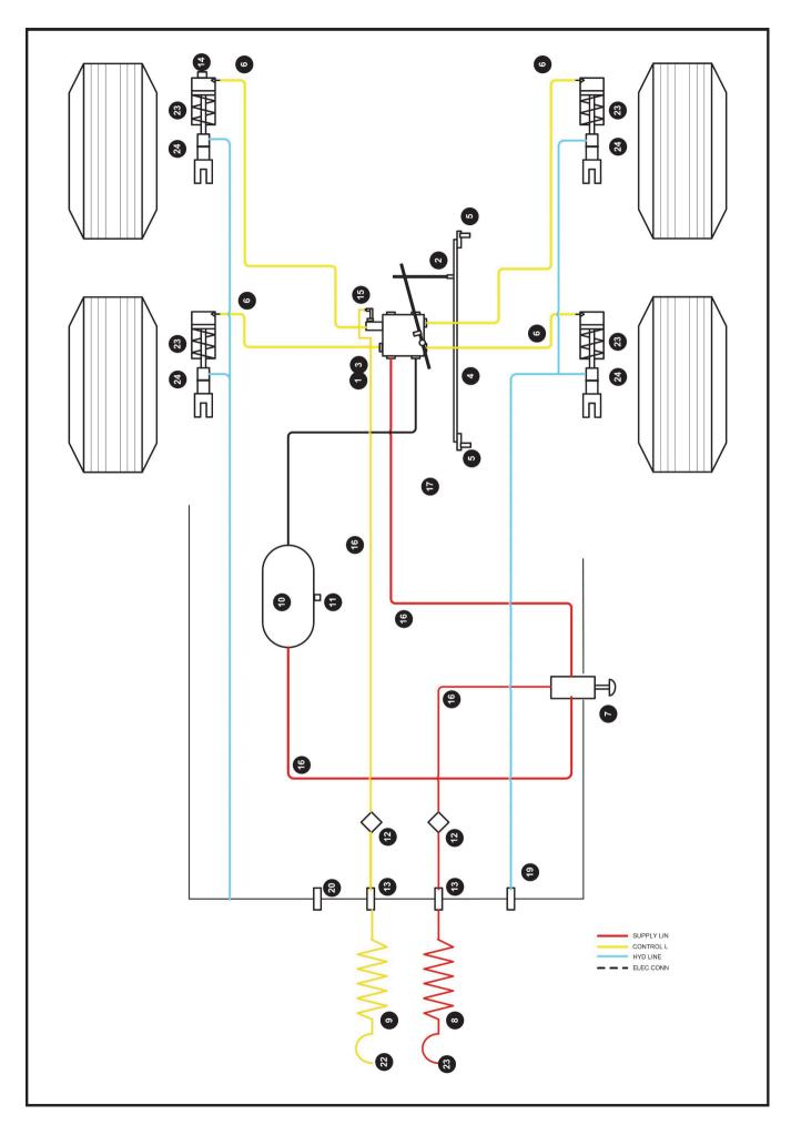
Two Line Air / Hydraulic with Mechanical Load Sensing Valve
