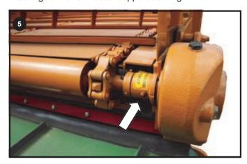
Grease Left Side Floor Drive shaft Support Bearings
