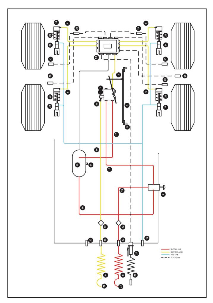
Two Line Air or Air / Hydraulic with Mechanical Load Sensing Valve & ABS
