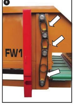
Grease all gear support bearings (4)
