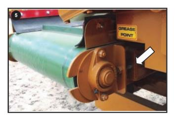
Adjust conveyor evenly to ensure accurate tracking Slacken the bearing location bolts on both sides of the conveyors left end., loosen the locknuts to the rear of the plate then by turning the threaded portion the locknut can be used to apply tension to the belt
