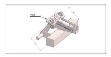
For braking systems which use a yoke, the yoke must remain parallel with the axle especially when the brakes are fully applied
