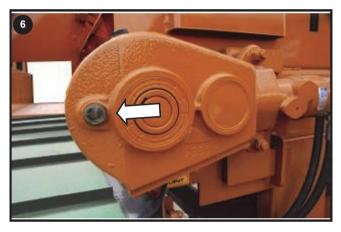
Check drive gearbox oil level. Replenish as required
