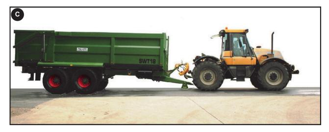
Hitching too low will cause unnecessary wear to the suspension and brake components of the front axle, and reduce the braking efficiency. It can also cause additional loading to be placed on the towing vehicle, possibly causing damage to rear axle and brake components.
