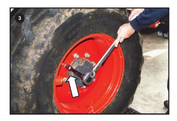
Check Wheel Nut Torque
