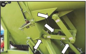
Grease Elevator linkage shafts
