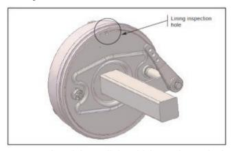
as the minimum lining thickness is reached.
