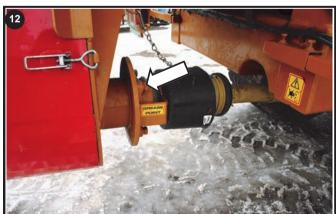
Grease Lower pulley shaft (Two positions)
