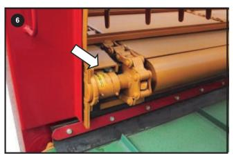
Grease Right Side Floor Drive shaft Support Bearings
