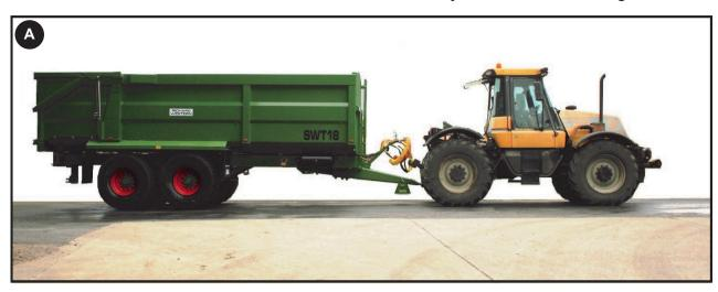
Adjust the drawbar and/or the hitch of the towing vehicle so that when towing the trailer body is parallel to the road surface.
