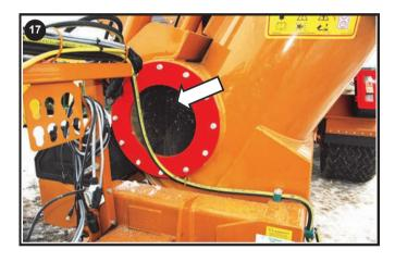
Grease Horizontal bearing (Via viewing window)
