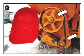
Grease Auger drive belt pulleys
