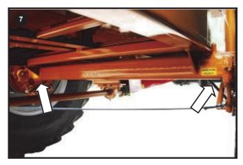
Grease Brake Actuators (Weekly)
