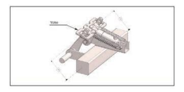
For braking systems which use a yoke, the yoke must remain parallel with the axle especially when the brakes are fully applied
