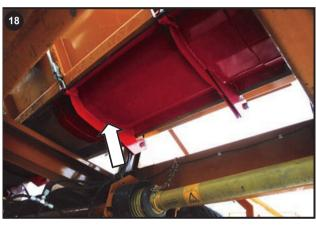
Grease Mid Auger bearing (Open Clear out hatch)
