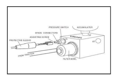
Note! The pressure switch is factory set and sealed. If seal is broken warranty for the unit becomes void.
