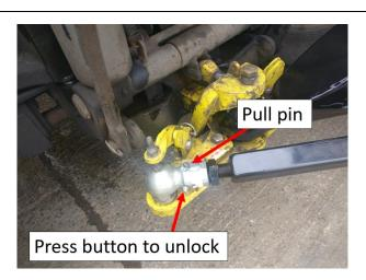
✓ Turn tractor & trailer slowly so latching mechanism lever pops back in as shown
