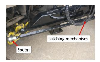
✓ Be sure spoon is attached correctly by pulling the pin and pressing the button at the side.
