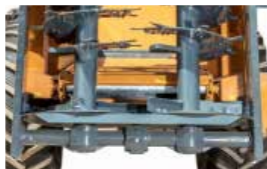
1.7m or 2.0m wide rotor spreading deck depending on model
