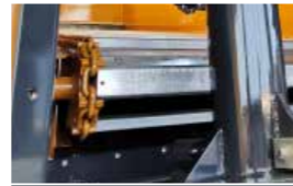
65mm or 80mm floor drive shaft with 7 tooth self-cleaning sprockets
