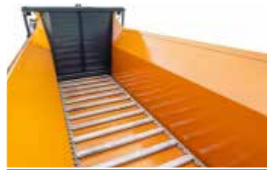
2 heavy-duty floor chains with individual tensioning, 16mm or 20mm, floor slats every 5 links
