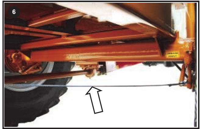
Grease Drive shaft Support Bearings
