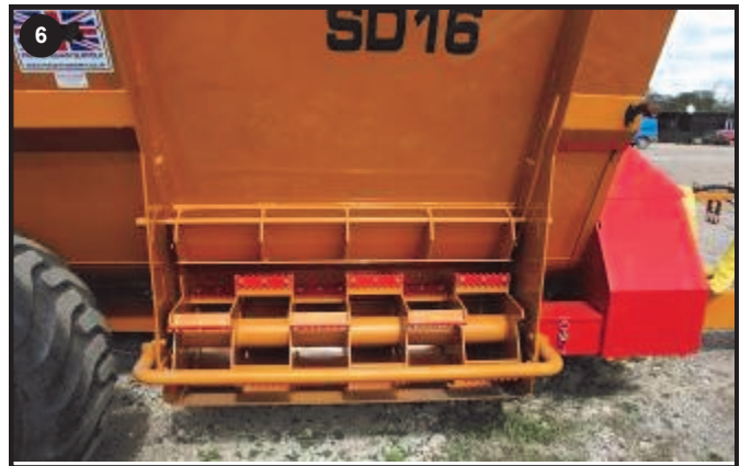
Replace the rotor blades when they become worn to prevent damage to auger See procedure below.
