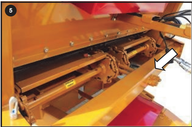
Adjust Floor chains. To give equal tension on each chain. When lifted in the centre of the body there should be approx. 100mm free play.
