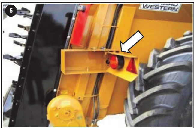
Check Lights & Reflectors for Correct operation & Damage
