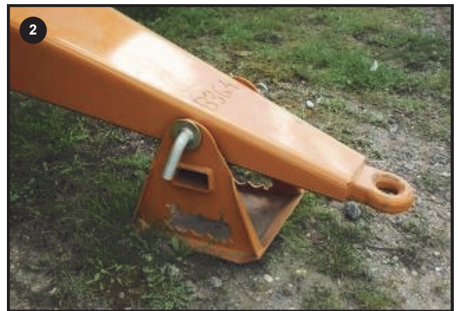
Check the condition of the Towing eye for signs of wear or damage
