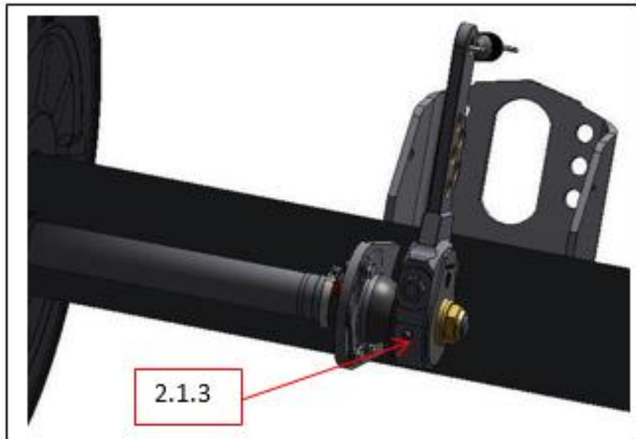
Figure 9 Showing Grease Point on Slack Adjuster
